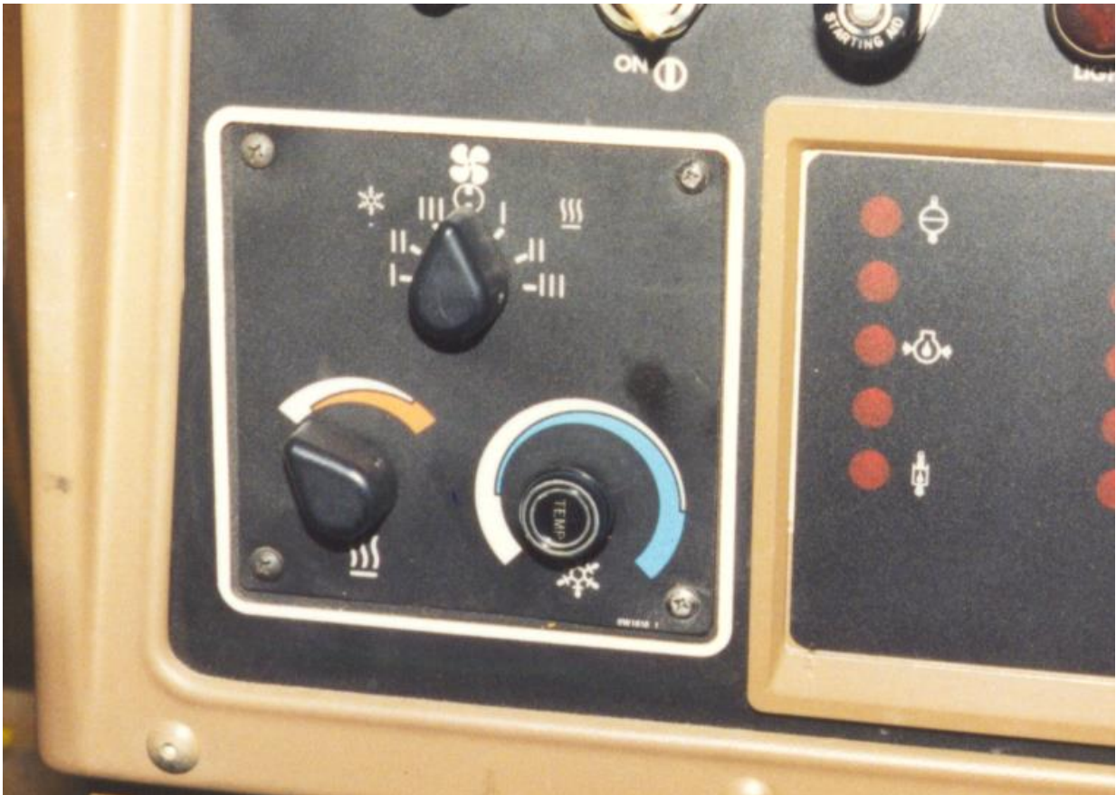
Thermostat in location on dash control panel.
